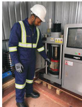
Samuel Mugo, a Civil Engineering student, works on an automatic concrete compression machine during his industrial attachment.
