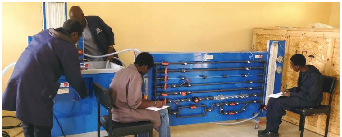
Engineering Students during a Laboratory Session using a Pipe Friction Loss Apparatus with a Hydraulic Bench.
